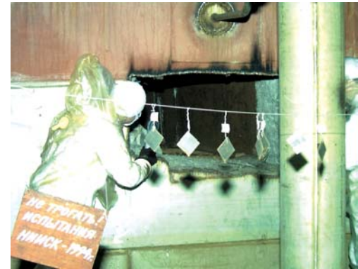
Examining the condition of engineering structures of the Shelter Object
