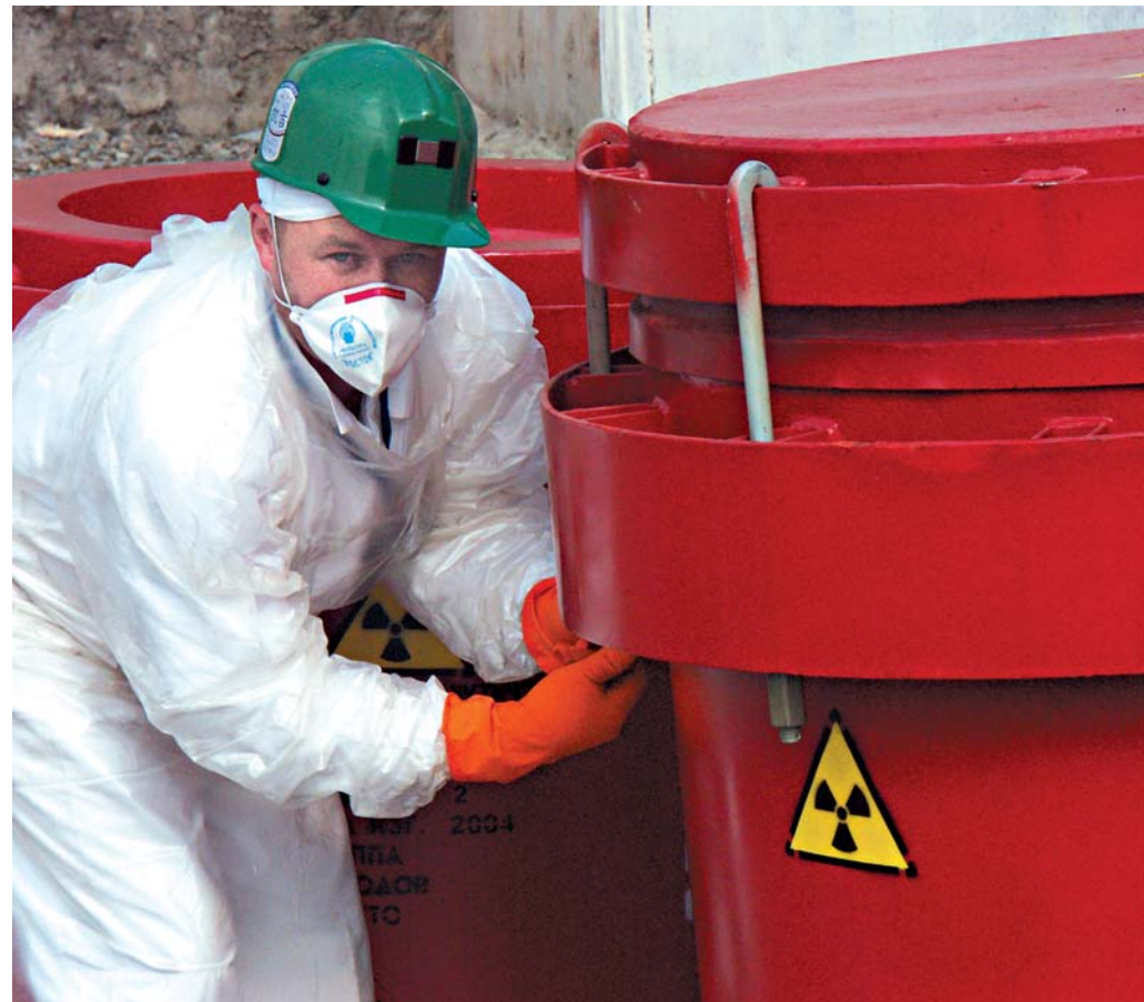
Special containers used for packaging radioactive waste
